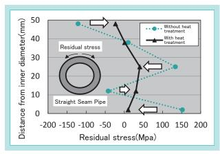
Fig. 7 Stress Relief by Annealing
