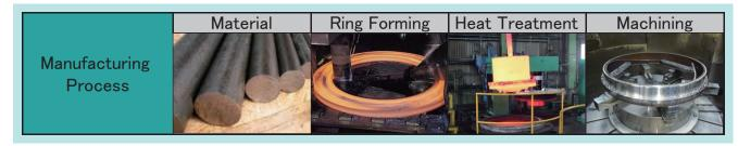
Fig. 2 Manufacturing Process of a Mechanical Joint
