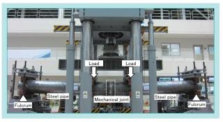
Fig. 10 Four Point Bending Test of Mechanical Joint(1)
