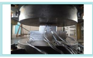
Fig. 9 Bearing Pressure Test of the Load Transfer Key
