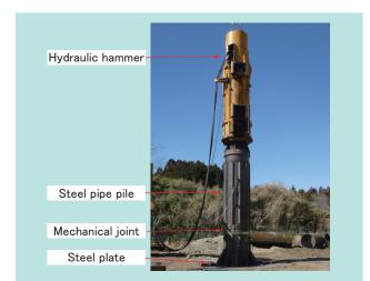
Fig. 12 Repeat Impact Test with a Hydraulic Hammer
