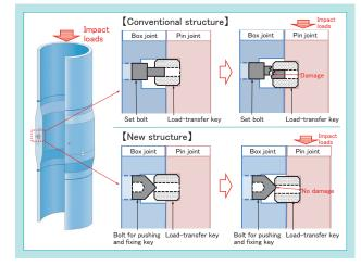
Fig. 14 Improvement of the Fixing Method
