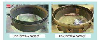
Fig. 13 Mechanical Joint After a Repeat Impact Test
