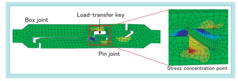
Fig. 8 Stress Concentration Zone of a Mechanical Joint
