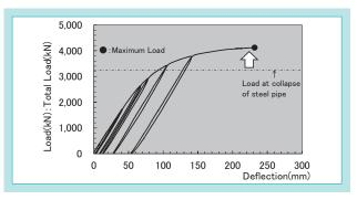
Fig. 11 Four Point Bending Test of Mechanical Joint(2)
