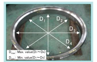
Fig. 6 Measurement Position of Roundness
