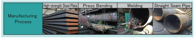
Fig. 3 Manufacturing Process of a Straight Seam Pipe
