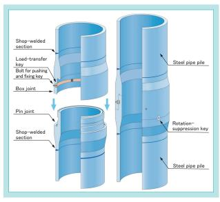
Fig. 1 Mechanical Joint (Laquican Joint)
