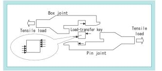
Fig. 4 Force Transfer Mechanism of a Mechanical Joint
